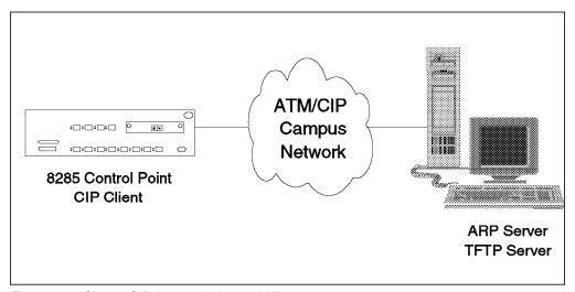
Figure 39. Simple CIP Network - Logical View
